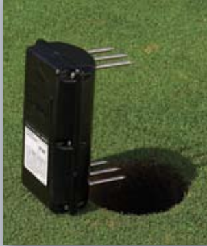
Wireless Sensor Measures Moisture, Temperature and Salinity Levels
